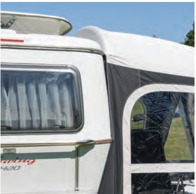
Optional Eriba Weather Protection Strip prevents rain running into the gully between the caravan and awning.
